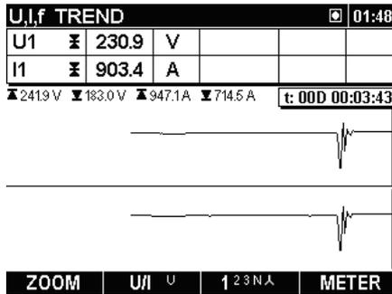
Figure 3.11: Voltage and current trend (dual mode)
