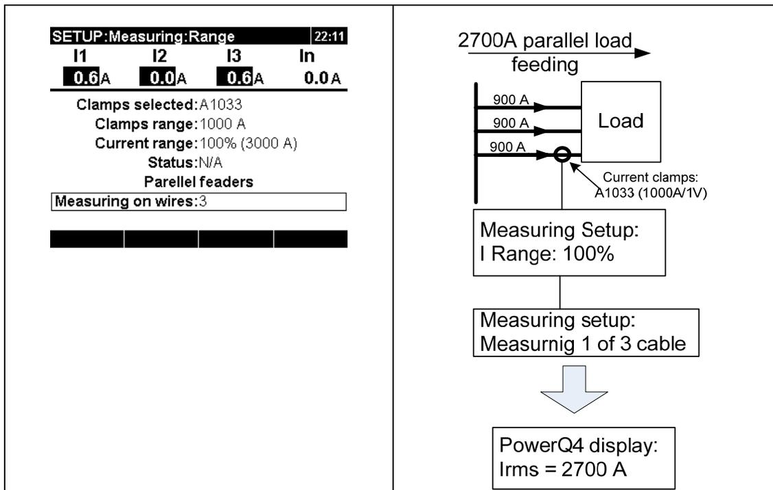
Figure 4.10: Parallel feeding of large load
