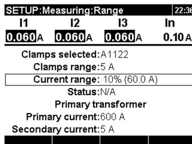
Figure 4.12: Selecting 10% of current clamps
