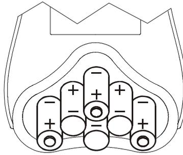
Figure 6.1: Battery placement
