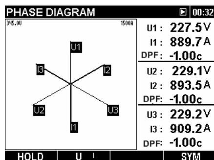
Figure 3.32: Phase diagram screen.
