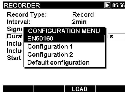
Figure 5.12: Predefined EN50160 recorder configuration
