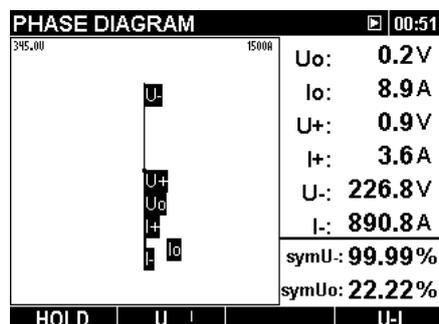
Figure 3.33: Symmetry diagram screen
