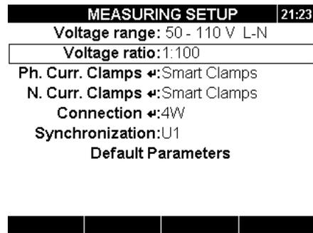
Figure 4.8: Voltage ratio for 11kV/110kV transformer example
