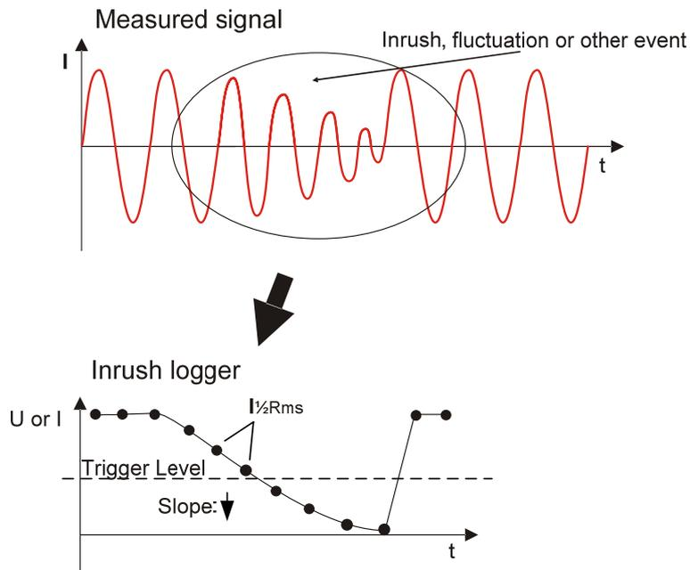
Figure 5.10: Inrush (waveform and RMS)
