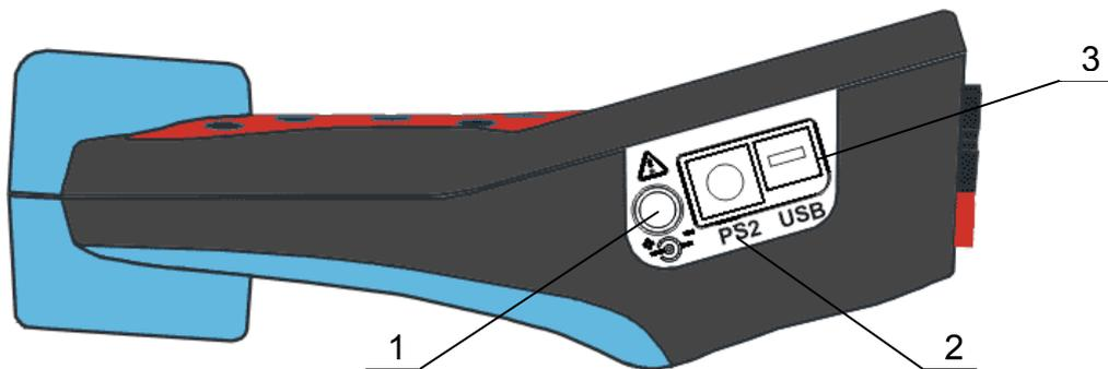
Figure 2.3: Side connector panel
