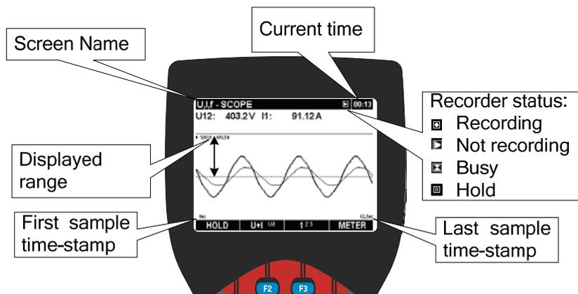
Figure 3.2: Common display symbols and labels during measurement campaign
