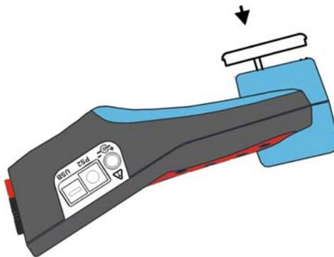
Figure 6.2: Closing the battery holder
