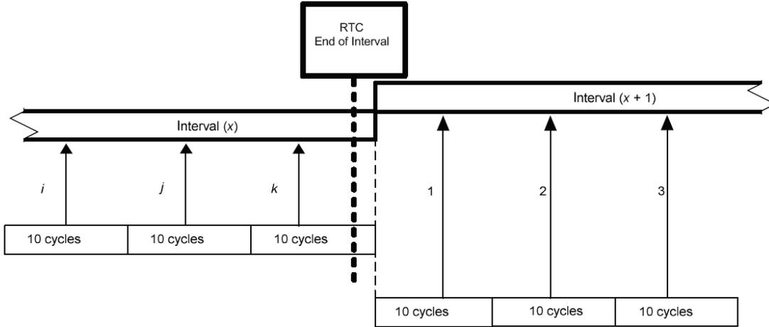
Figure 5.9: Synchronization and aggregation of 10 cycle intervals
