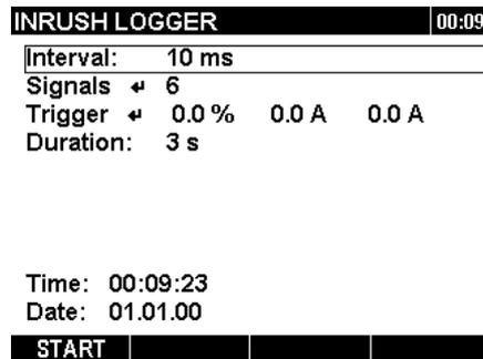
Figure 3.24: Inrush logger setup screens.
