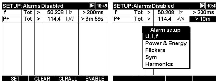
Figure 3.42: Alarms setup screen.
