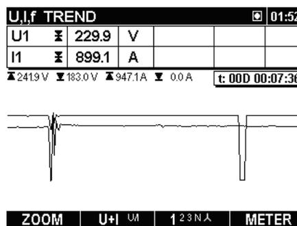
Figure 3.10: Voltage and current trend (single mode)
