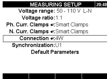
Figure 4.1: Measuring configuration menu
