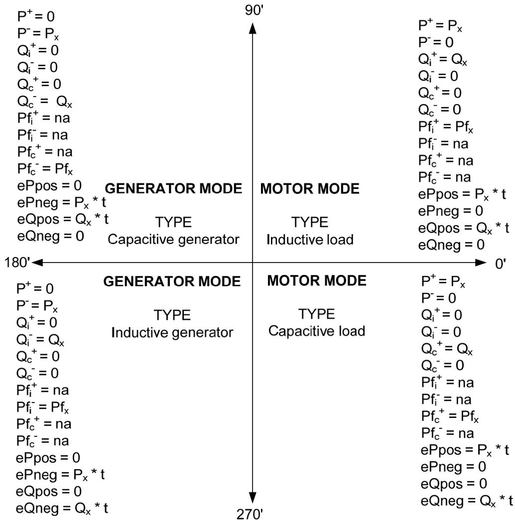
Figure 1: Motor/generator and inductive/capacitive phase/polarity diagram
